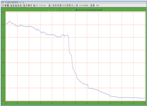
图 4 全省 10 kV 分布式光伏实际调节曲线 Fig.4 Actual adjustment curve of 10 kV distributed photovoltaic in the whole province
